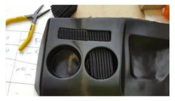
Following the completion of printing, the part will be post-processed to the client's requirements. This includes removing any supports and can be as simple as a quick sanding to smooth a part or can involve full painting for immediate use in a car.
