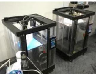
Many parts that are requested are for external use on the vehicle. Items like a 6ft spoiler, are too large to complete on a single printer. Using ideaMaker, Big Bear is able to split his model into 7-8 interlocking pieces and delegate the print jobs to his fleet of N2 and N2 Plus printers. By delegating the work to multiple printers and printing simultaneously, the turnaround time for each product is greatly reduced.
