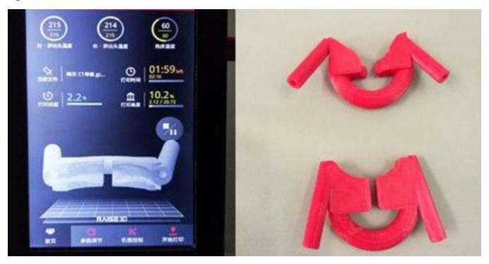
In software, Niu's team designs these models with tubes or canals that will guide the drill holes. These holes are designed at specific angles, lengths, and diameters to precisely match up with the desired outcome and the surgery tools that will be used. The team will test the printed guide on the observation model and adjust the model if necessary; guaranteeing a perfect fit.
